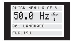
At the bottom of the display, the parameter number and name are given together with the status/value of the first parameter under Quick Setup. The first time the [Quick Menu] key is pressed after the unit has been switched on, the read-outs will always start at pos. 1 - see table below.
