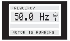
Line 2 gives the data value of an operating variable with related unit, and line 1 provides a text which explains line 2, cf. table. In the example, Frequency has been selected as variable via parameter 009. During normal operation another variable can immediately be read out by using the [+/-] keys.
