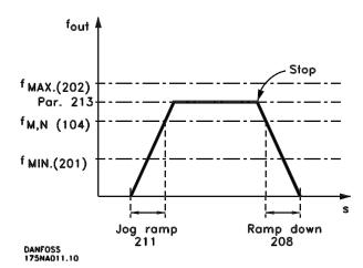
The jog ramp time starts if a jog signal is given via the digital inputs or the serial communication port.
