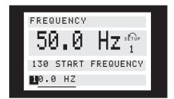
The chosen digit is indicated by the digit flashing. The bottom display line shows the data value that will be entered (saved) when signing off with [OK].
