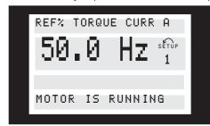
This is where parameter names and units for operating variables in the first line are given - operating variable 2 remains unchanged.
