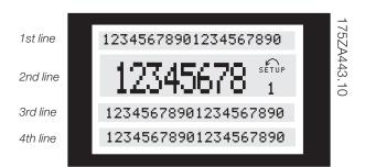
**1st line** shows up to 3 measurements continuously in normal operating status or a text which explains the 2nd line.
