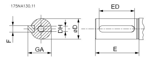
Shaft tapped DH x deep to DIN 332 Form DR Closed profile keyway
