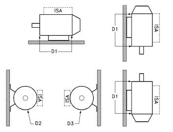
D1: Drain holes opposite inverter side, both drive end and non drive end. D2/D3: Drain holes 90° to inverter, both drive end and non drive end.
