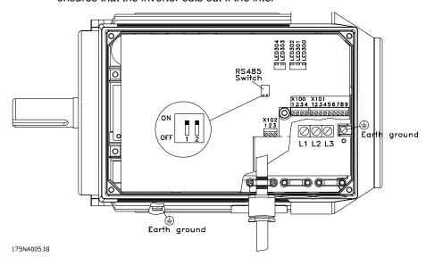
Terminal arrangement (for installation see quick setup, MG.03.AX.62)
