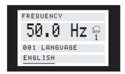
The bottom display line shows the text value that will be entered (saved) when acknowledgement is given [OK].
