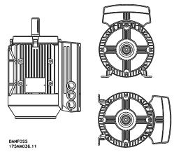
FC motors must be installed with adequate access for routine maintenance. A minimum of 0.75m of working space around the motor is recommended. Adequate space around the motor, particularly at the fan inlet (50 mm), is also necessary to facilitate airflow.
