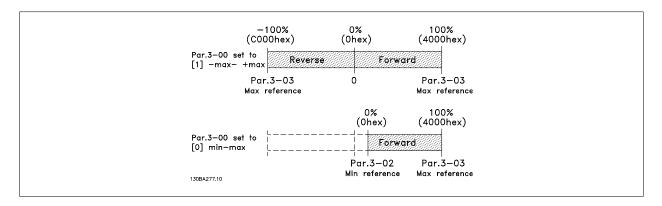
The actual reference [Ref. %] in the VLT frequency converter depends on the settings in the following parameters:
