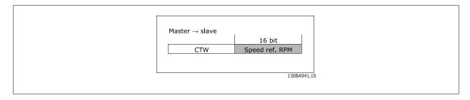
The speed reference value should be transmitted to the VLT frequency converter in the form of a 16-bit word. The value is transmitted directly in RPM.
