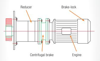
The EC centrifugal brakes consist essentially of a **central core that rotates integrally with the motor shaft**. On its periphery a series of masses are distributed among sectors. These masses are carried by the guides.
