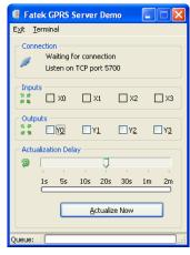
*Details:* Program listens on TCP port 5700 for incoming connection. Port 5700 is default port where FBs-CMGSM connects to. Program periodically queries status of inputs X0-X3 from remote station. You can change any of output Y0-Y3 by click on a check box Y0-Y1.
