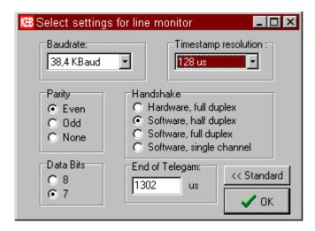
Following adjustments are possible for the telegram end identification (Handshake):
