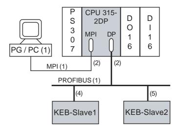
**5.1 Setup of Test Environments** To carry out the test of the driver the above shown test setup is necessary. Generally two possibilities for the PROFIBUS-coupling of KEB-units is possible. The following gives a short description of the necessary configuration for both:
