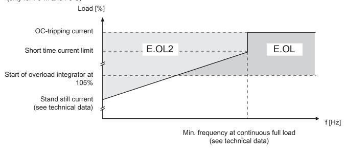
A PT1-element ( $\tau$ =280 ms) starts if the permissible current is exceeded. After its sequence of operation error E.OL2 is triggered.
