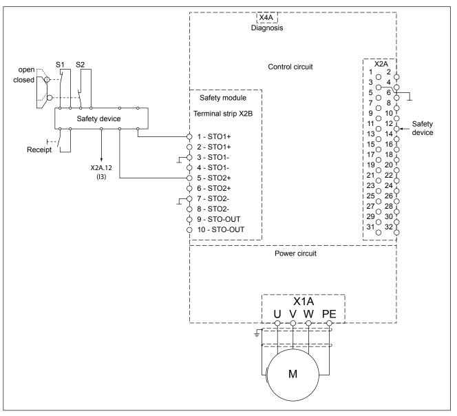
When pressing the emergency stop unit the drive is stopped with a deceleration ramp via input X2A.12 (I3).
