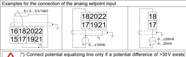
Connect potential equalizing line only if a potential difference of >30V exists between the controls. The internal resistance is reduced to 30kΩ.
