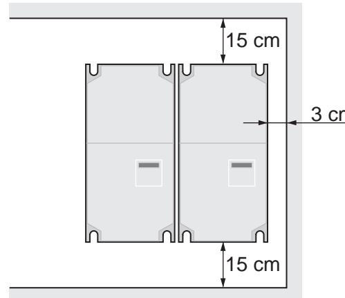
15 cm min. distance at air inlet and air outlet to the next subassembly
