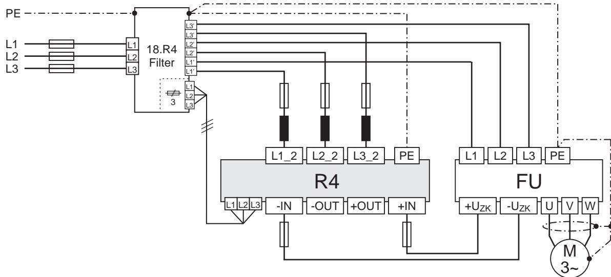
**FU > Size 17 ( $I_{max} > 45$  A, for correct dimension of R4)**
