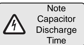
Before any installation and connection work, the system must be switched off and secured.
