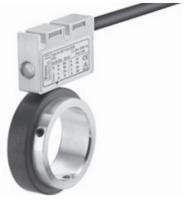
Thanks to its installation depth of only 16 mm, the bearingless magnetic rotary encoder RI20 / LI20, comprising a magnetic ring and sensor head, is ideally suited for plants and machinery where space is very tight. The non-contact measuring principle allows for error-free use even under harsh environmental conditions, as well as ensuring a long service life.
