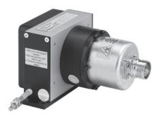
These draw wire mechanics can be combined with all encoders having a size 58 synchro flange and 6 mm shaft.
