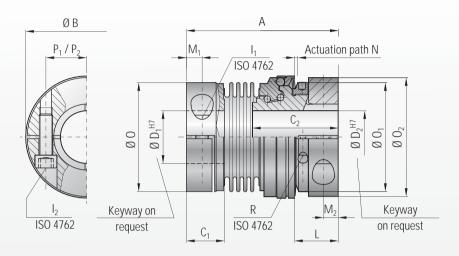
Clamping hub with one ISO 4762 screw per hub. Components of compact and rigid design with backlash free interface. Misalignment compensation via torsionally rigid bellows
