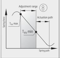
Attention! R+W safety couplings have disc springs with a special characteristic. The torque adjustment range lies within a specific range of positions for the disc spring, outside of which the torque limiter can not function. It is important to always stay within the min. — max. of the specified torque adjustment range.
