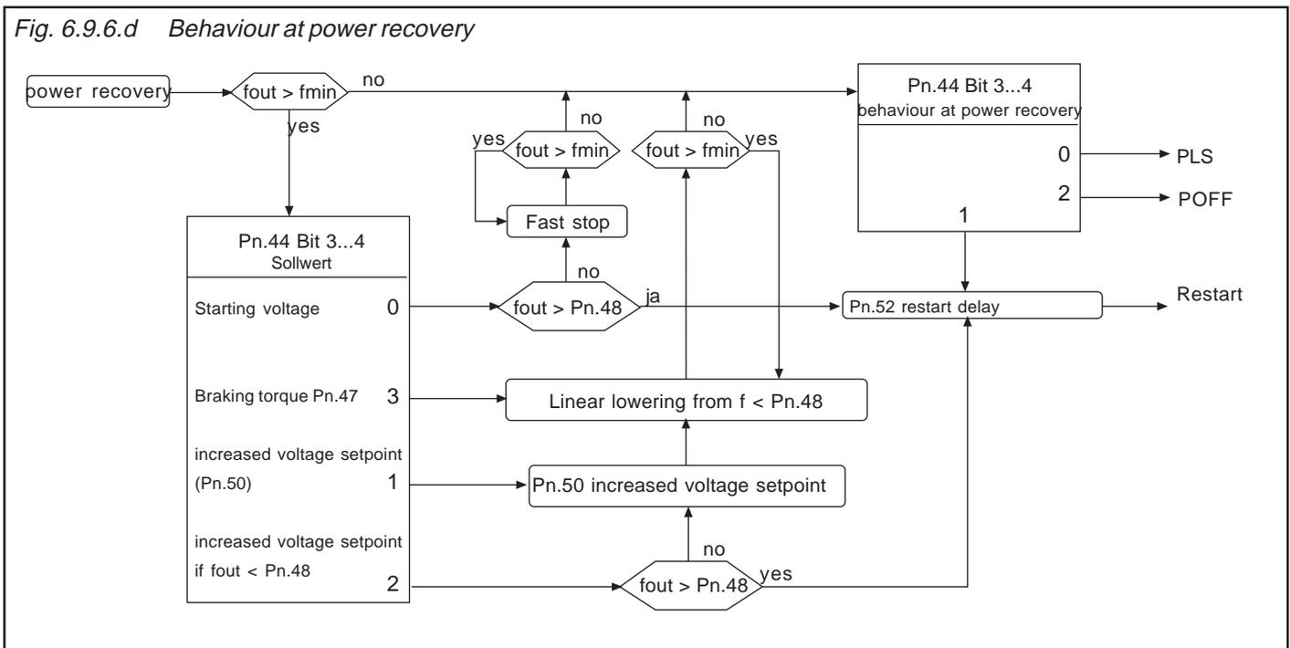
Behaviour at power recovery The following parameters effect the behaviour of the inverter if the system voltage returns during the Power-Off-function
