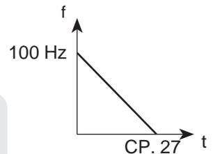
Example: actual deceleration time = 5s; the drive should decelerate from 50 Hz to 0 Hz. delta f = 50 Hz - 0 Hz = 50 Hz
