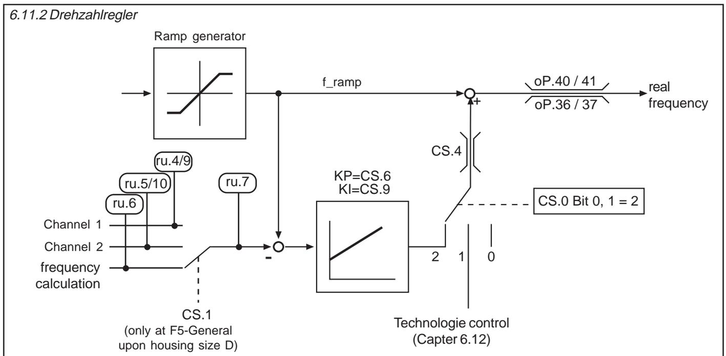
**Configuration speed controller (cS.0)**
