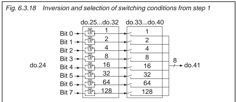
With the parameters do.25...do.32 each of the 8 flags (bit 0...7) from logic step 1 can be inverted separately. Through this function it is possible to set any chosen flag as Non-flag. The parameter is bit-coded. According to Fig. 6.3.18 the weighting of the switching conditions to be inverted must be entered in do.25...do.32. If several flags shall be inverted, the sum is to be formed.
