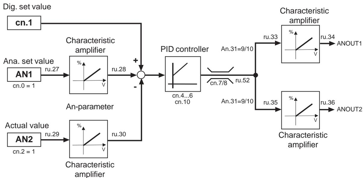
**PID-Controller as active current- (torque-) regulation without precontrol**
