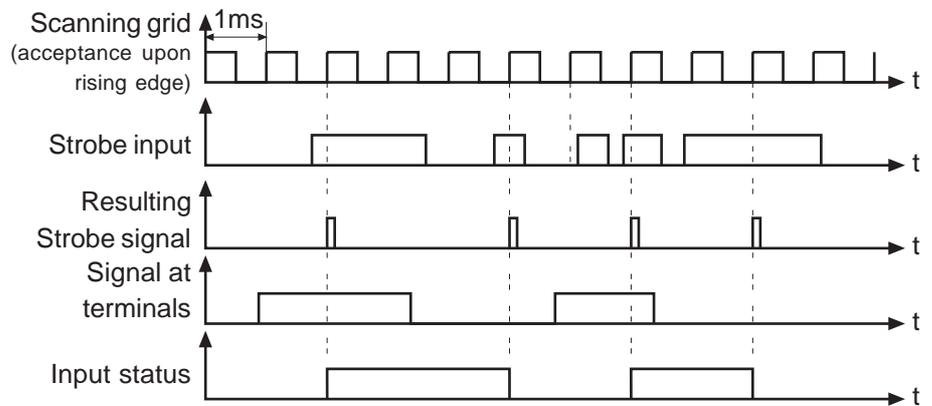
Fig. 6.3.8.b Static Strobe Mode 1 (di.7=1)
