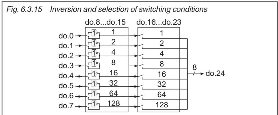
With the parameters do.8...do.15 each of the 8 switching conditions (do.0...do.7) can be inverted for each flag separately. Through this function it is possible to set any chosen switching condition as Non-condition. The parameter is bit-coded. According to Fig. 6.3.15 the weighting of the switching conditions to be inverted must be entered in do.8...do.15. If several conditions shall be inverted, the sum is to be formed.
