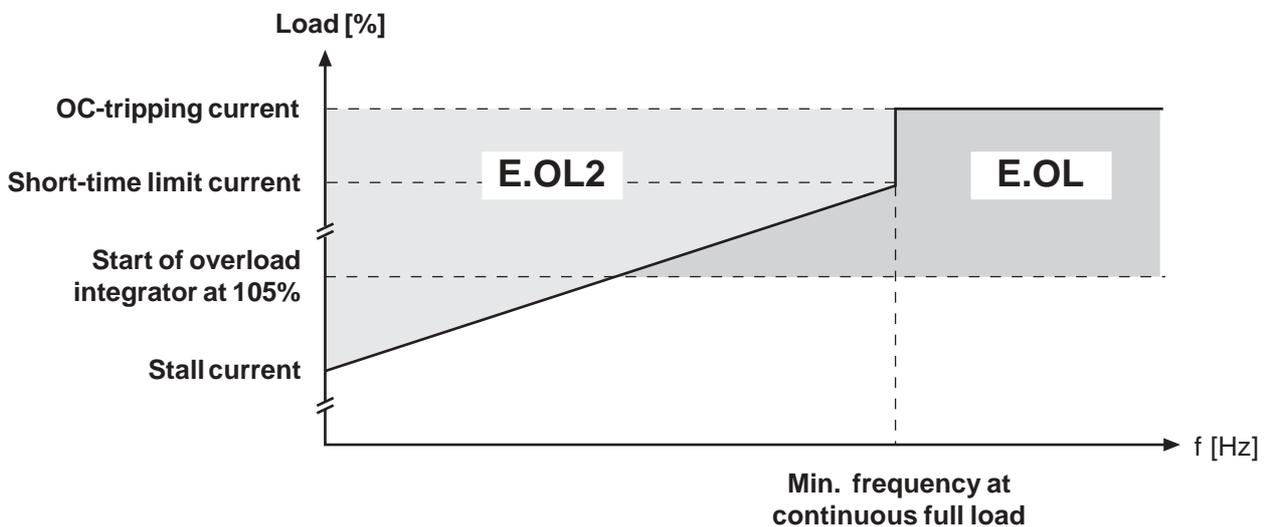
If the permissible current is exceeded a PT1-element ( $\tau=280\text{ms}$ ) starts, after its sequence of operation the error E.OL2 is triggered.
