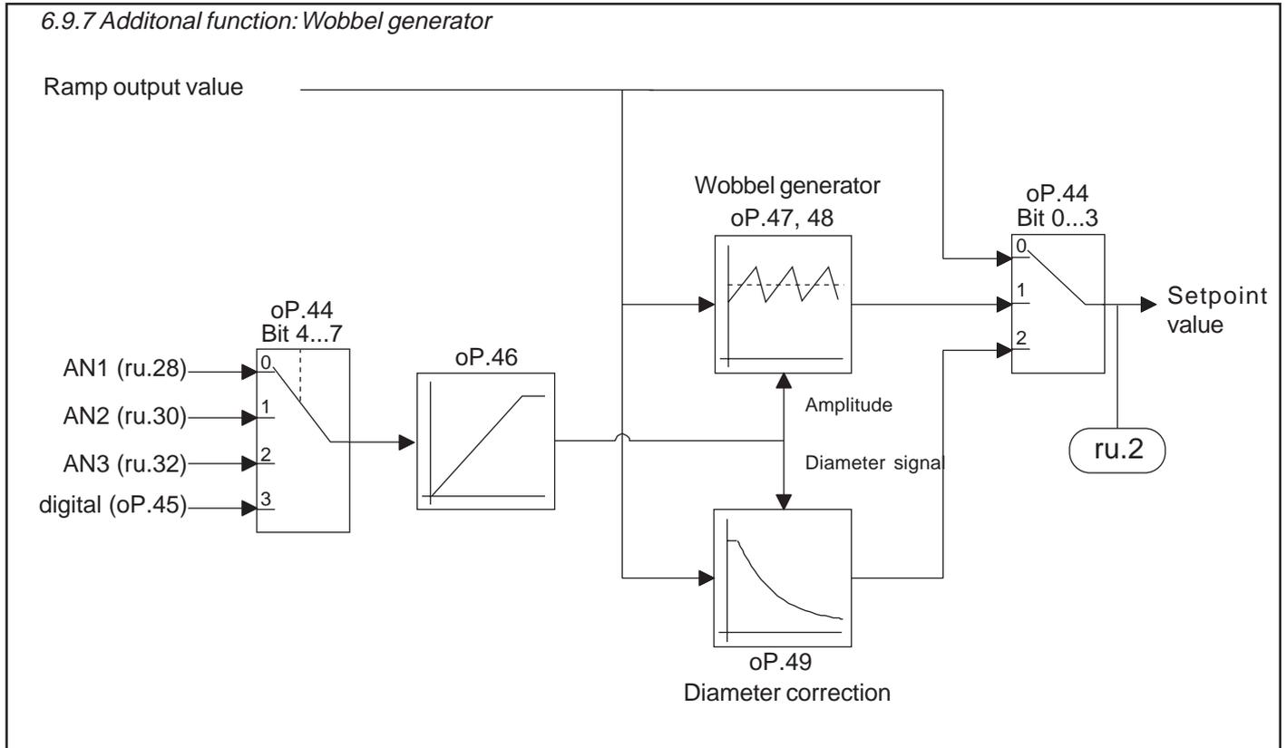
Additional function/ Mode (oP.44 Bit 0...3) Different functions can be activated with oP.44 Bit 0...3. The value is to be added to Bit 4...7.
