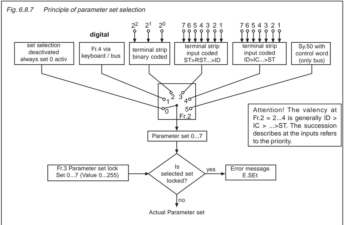
Fr.2 Source parameter set As shown in Fig. 6.8.7, with Fr.2 it is defined whether the parameter set selection is enabled or disabled via keyboard/Bus (Fr.4), the terminal strip or via control word (SY.50). The selection is activated with „Enter“.
