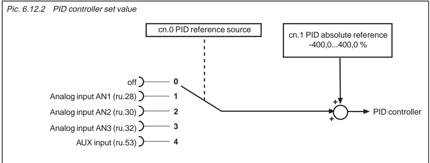
**PID absolute reference (cn.1)** With cn.1 the set value of the PID-Controller is preset digitally in the range of -400,0...400,0%. The parameter is set-programmable.
