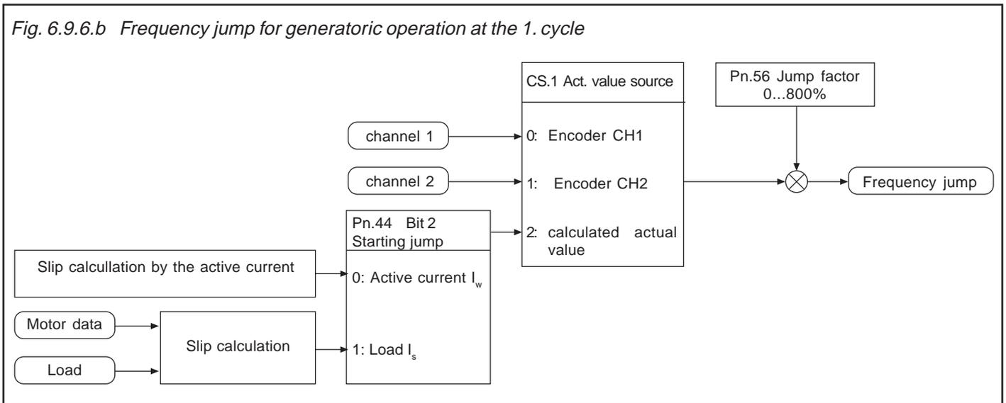
**Frequency jump for generatoric operation** First of all the drive must be brought into generatoric operation to enable the feed back of energy into the intermediate circuit. This is achieved by making a frequency jump, so that the speed of the drive is larger than the output rotating field speed of the inverter.
