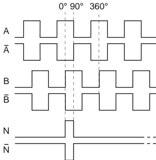
The two, by 90° electrical out of phase signals, A and B as well as their inverted signals are generally evaluated. The zero track is needed for the reference point approach in the positioning module (F5-M/S). Zero track (also reference marking channel) gives out 1 signal per revolution.
