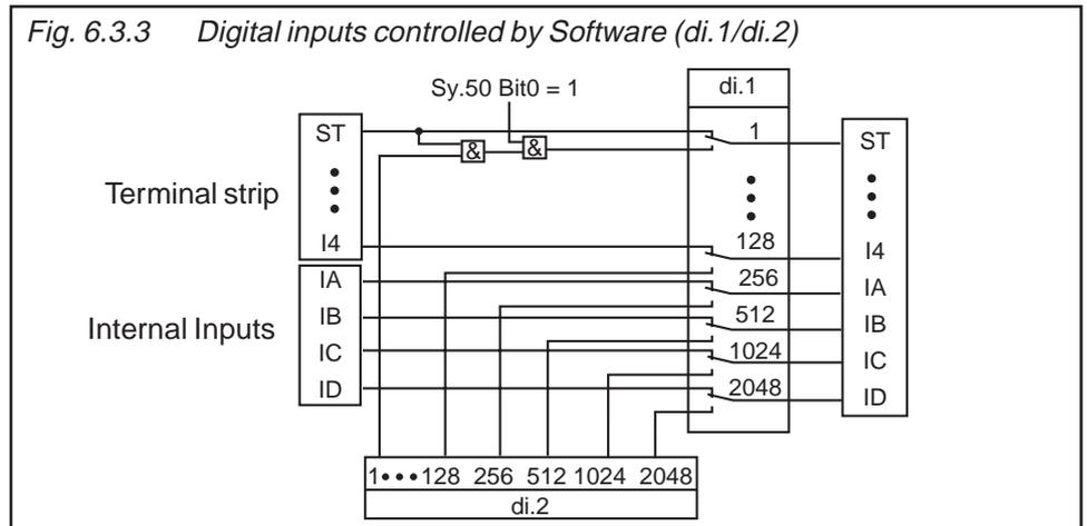
As shown in Fig. 6.3.3, it can be selected with di.1, whether the inputs shall be switched from the terminal strip (default) or by way of parameter di.2. Both parameters are bit-coded, i.e. according to following table, the appropriate value for the input is to be entered. In the case of several inputs the sum is to be formed. (Exception: Control release must always be bridged at the terminal strip).
