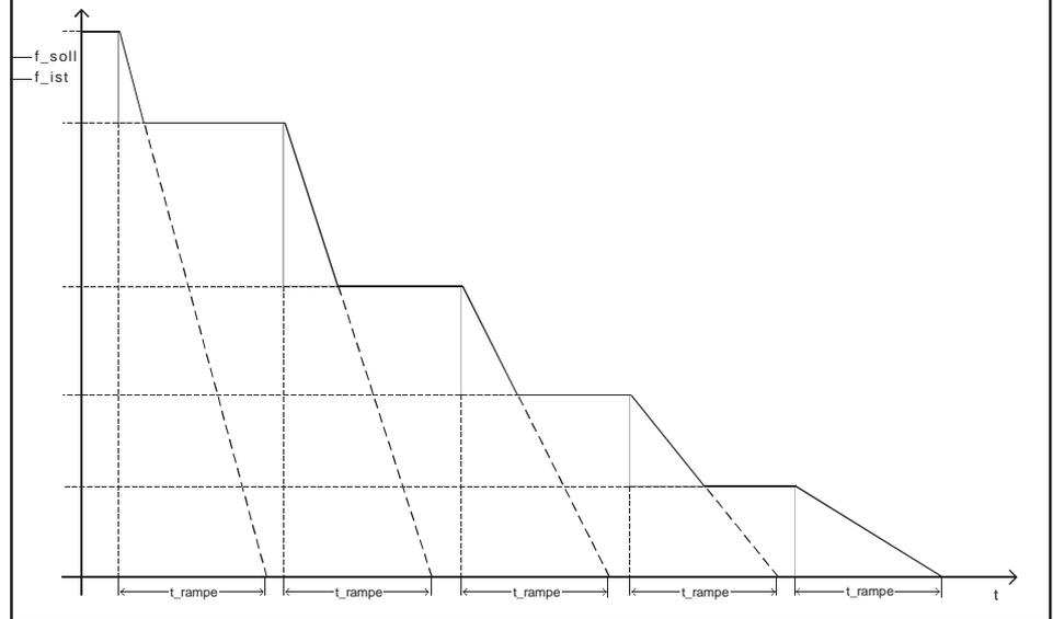
**Ramp mode (oP.27)** The different ramp functions can be adjusted separately for every frequency change (acceleration forward, deceleration forward and so on). The selection is made with oP.27 and is adjustable separately in each set. The function is activated after pressing „ENTER“.
