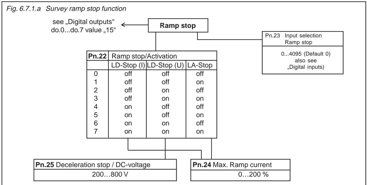
**LA-Stop** The function protects the frequency inverter against switch off caused by overcurrent during the acceleration phase. The current level is adjustable with Pn.24 in the range of 0...200 %. The protective function can be deactivated with Pn.22.
