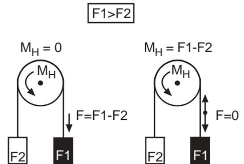
Fig. 6.9.5.b Principle of brake control
