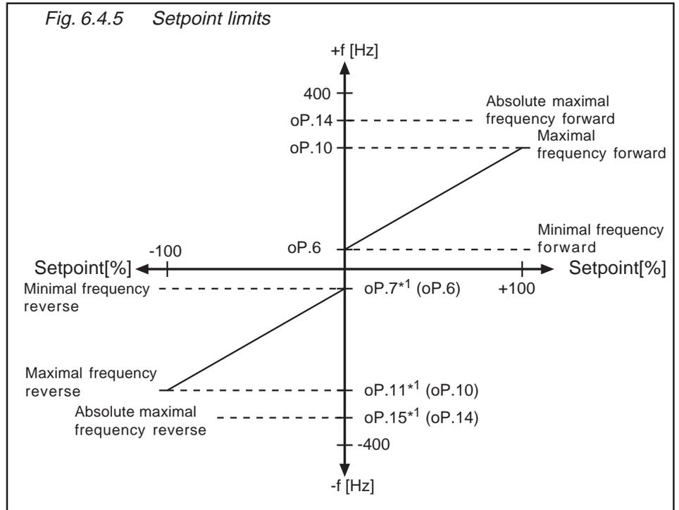
\*1 If the value „=For“ is adjusted in these parameters (limit values rotation direction reverse), then the adjusted values for rotation direction forward (oP.6, oP.10 and oP.14) are valid.
