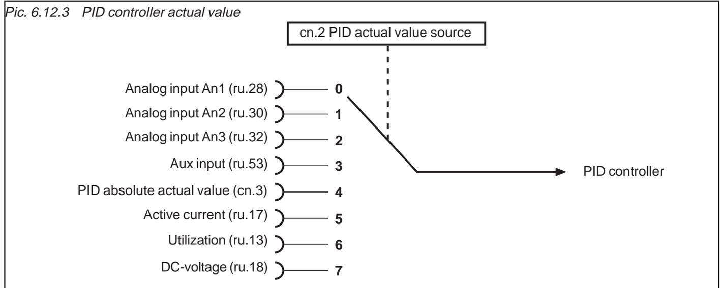
PID actual value source (cn.2) The actual value source (cn.2) determines from where the PID-Controller receives the actual value signal. Following signals are available:
