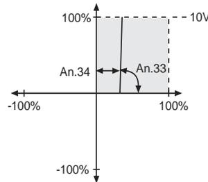
Because of the high amplification the analog output switches in a relative small switching window.
