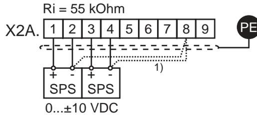
1) Connect equipotential bonding conductor only, if a potential difference of > 30V exists between the controls. The internal resistance is reduced to 30 kOhm.
