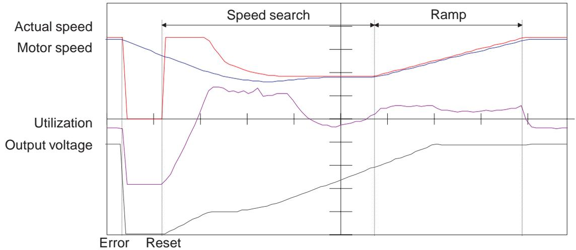
Fig. 6.7.3.c Speed search with „fast“ adjusted function
