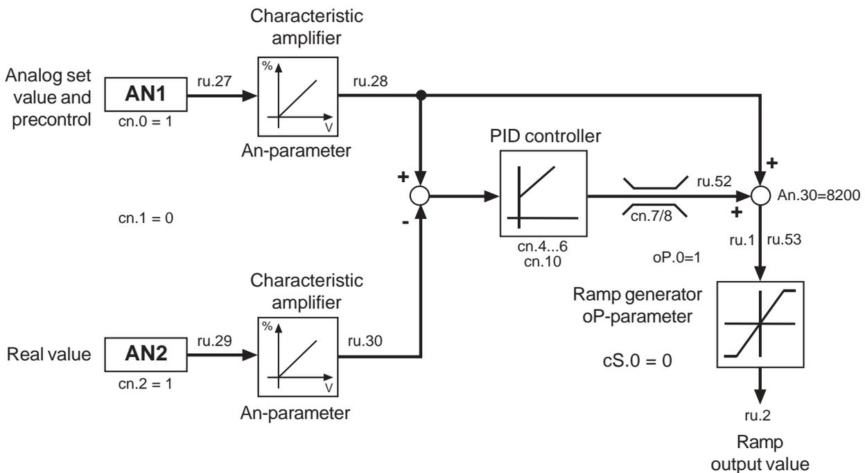
**PID-Controller on the analog output**
