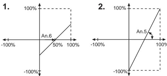
With these settings the entire speed range can be driven with 0...10 V via input AN1.
