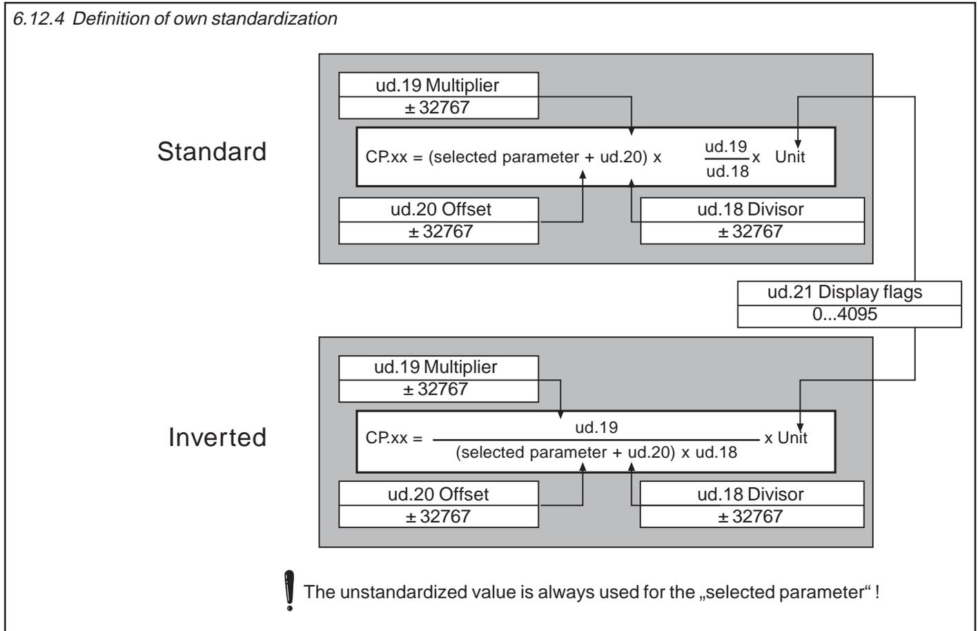
**ud.18 Display standardization Divisor** Adjusts the divisor in the range of ±32767 (default 1). The parameter is set-programmable (not at B-control).
