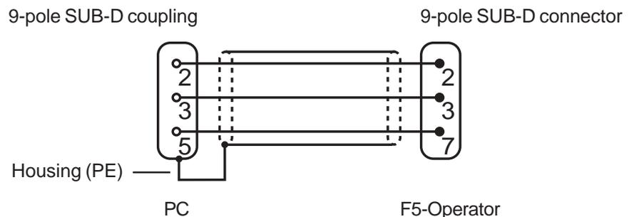
**!** The RS232-cable is suitable exclusively for the communication between PC and Operator. If the cable is plugged in directly onto the control board, it can lead to the destruction of the interface of the PC.
