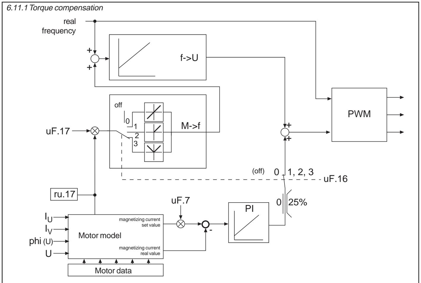
**Motordata** The motor data is entered in the parameters dr.0...dr.6 as described in Chapter 6.6.
