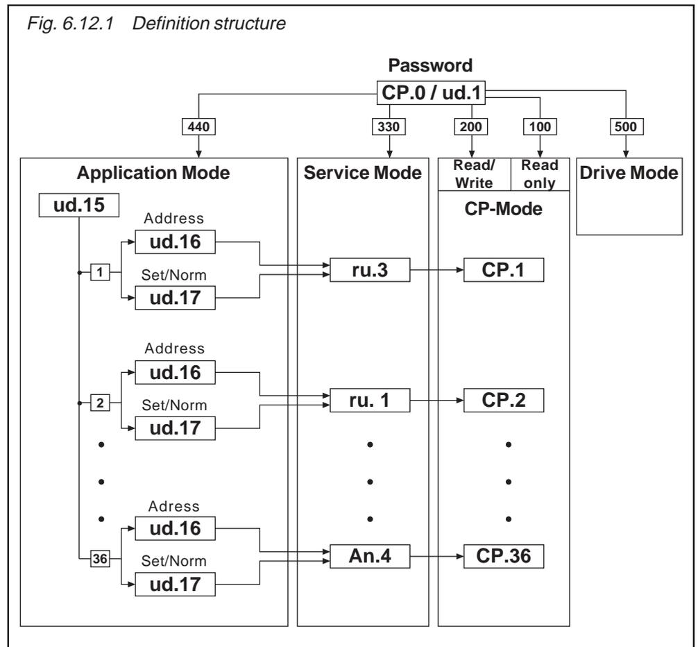
With ud.15 the CP-parameter that is to be edited is determined. With ud.16 and ud.17 the CP-parameter is defined through its address and the respective set. Depending on the adjusted password (CP.0 or ud.1)
