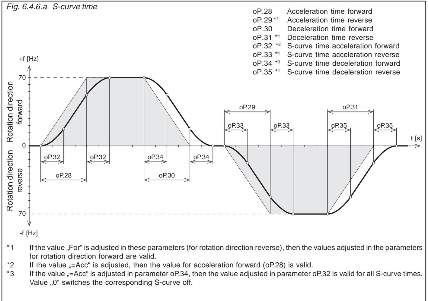
! In order to drive defined ramps with activated S-curve time, the preadjusted acceleration and deceleration times (oP.28...oP.31) must be larger than the S-curve time (oP.32...oP.34) belonging to it. !
