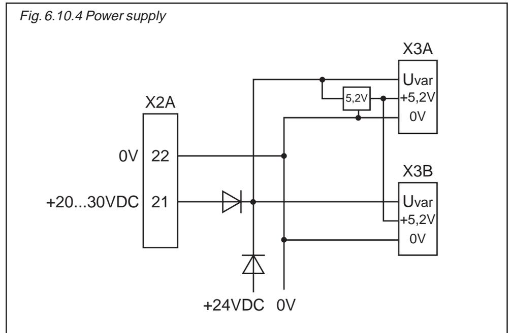
**U<sub>var</sub>** U<sub>var</sub> is an unstabilized voltage that is provided by the power stage of the KEB COMBIVERT. Dependent on the size of unit and the load, the voltage amounted to 15... 30 V DC. Uvar is loadable at X3A and X3B with altogether 170 mA. If higher voltages / currents to supply the encoders are needed then the control must be supplied with an external voltage.
