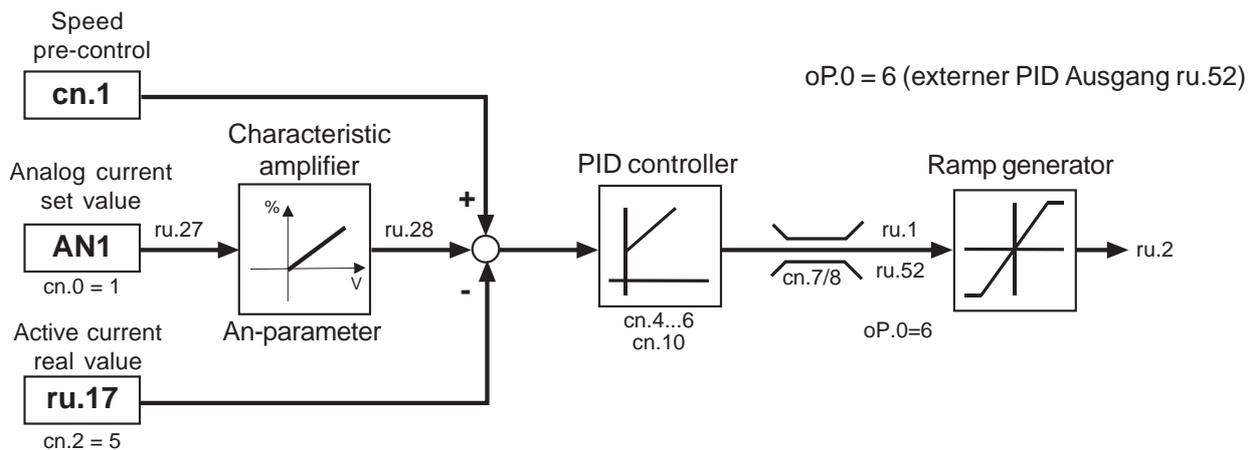
**PID-Controller as active current- (torque-) regulation without precontrol**
