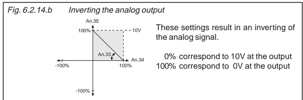
These settings result in an inverting of the analog signal.
