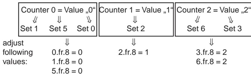
The counter works only in the active set with the measured value. In all inactive sets it is counted down. If one counter exceeds the limit, the response adjusted in Pn.14 is triggered.
