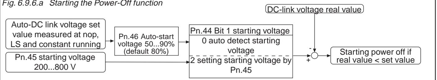
**Start voltage (Pn.45)** With manual adjustment the starting voltage can be preset with Pn.45 in the range of 200...800 volt. For a secure range the adjusted starting voltage must be at least 50 V over the UP-threshold (UP: 400V-class=280V; 200V-class=216V DC).
