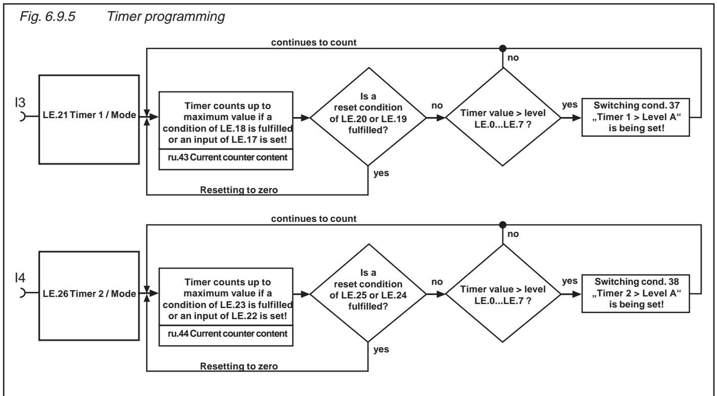
Timer / Mode (LE.21/26) LE.21 and LE.26 determine the clock source and the counting direction of timer 1 and timer 2. Clock source can be the time counter in 0.01 s or h-raster or impulses from an input. The timer runs generally as long as a starting condition is active. After a reset the timer starts again at zero. The timer stops at the maximal value of 655.35. Following clock sources can be selected:
