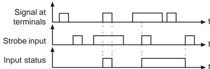
Fig. 6.3.8.c Static Strobe Mode 2 (di.7=2)
