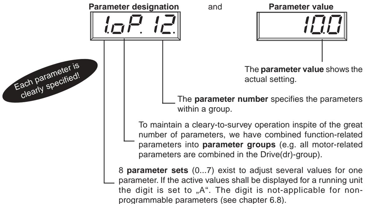
*Example:* A conveyor belt shall be used with 3 different speeds. A parameter set is programmed for each „speed“ ... acceleration, deceleration etc. can be adjusted individually.
