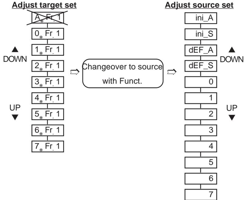
With the keys UP/DOWN and at flashing point the target set is adjusted in addition to the parameter set number. The active (A) parameter set must not be adjusted as target set while copying. If the target set is > 0, only the programmable parameters are overwritten!
