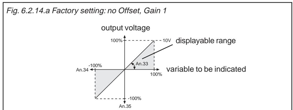
Inverting the analog output
