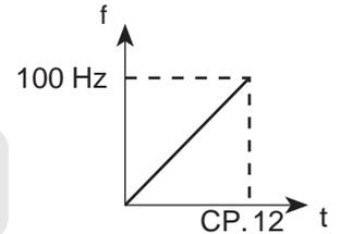
Example: actual acceleration time = 5s; the drive should accelerate from 10 Hz to 60 Hz.  $\Delta f = 60 \text{ Hz} - 10 \text{ Hz} = 50 \text{ Hz}$
