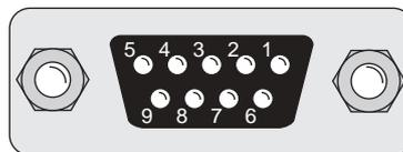
**! Only when the inverter is switched off and the voltage supply is disconnected may the plug be pulled out or plugged in!**
