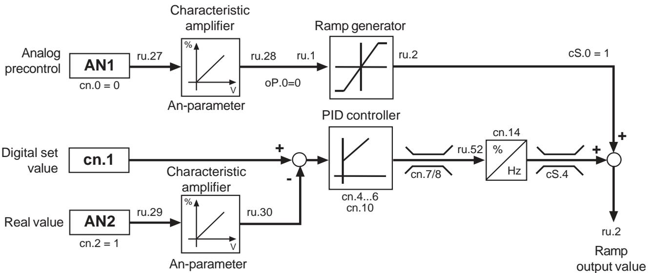
**PID-Controller with precontrol (Variant 3; e.g. for speed regulation with tacho generator - only for F5-G/B)**
