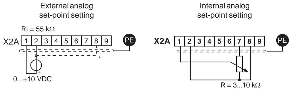
\*) Connect potential equalizing line only if a potential difference of > 30 V exists between the controls.
