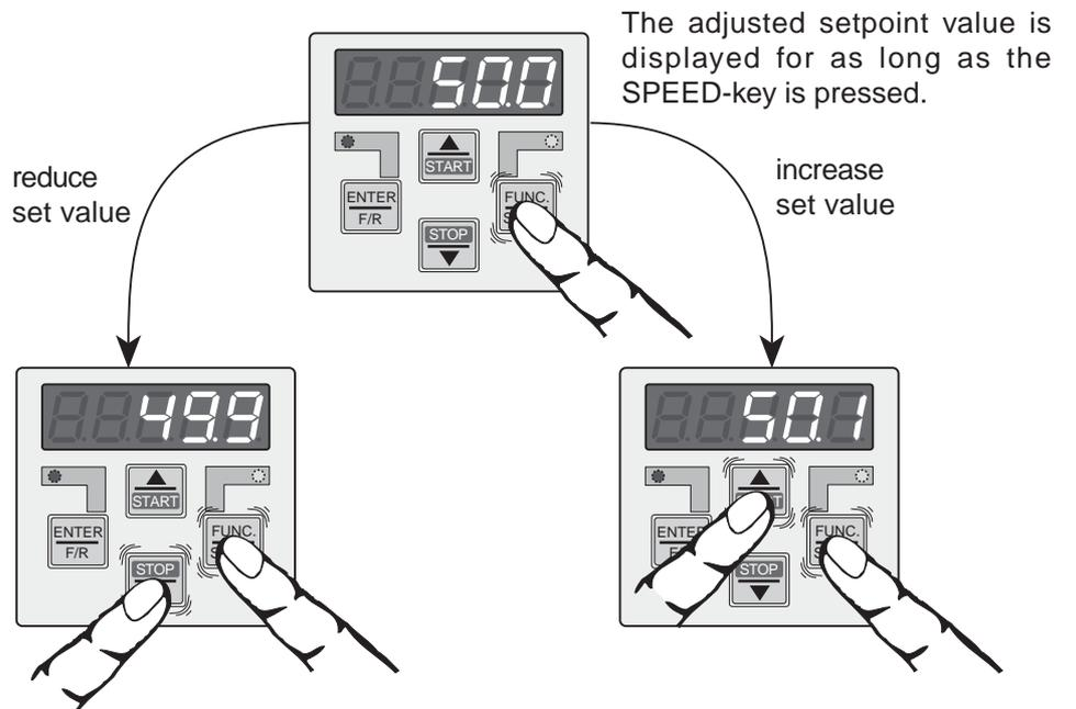
Press the SPEED-key and reduce the displayed setpoint value with the DOWN-key.
