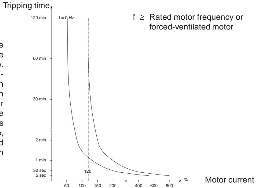
**Description for F5-S** The internal overload counter counts downwards (100 % to 0 % in 5 s) with overload factors < 300 %. Above 300 % it is counted upwards according to following characteristic.
